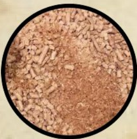
Caking Poor Quality Pellets
